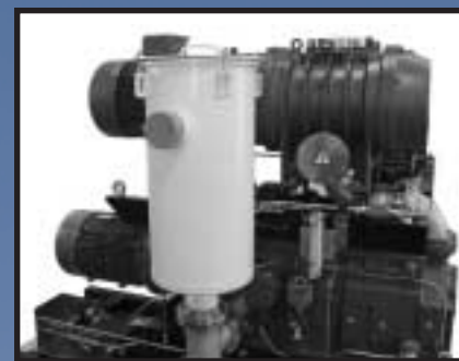
Severe Duty Exhaust Filter on Vacuum Pump
